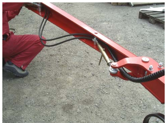
14. Mount the small turnbuckle and check that the spacer sleeves (A) are in place. Lock with tension pin (B). Knock the handle (C) through the hole in the turnbuckle.
