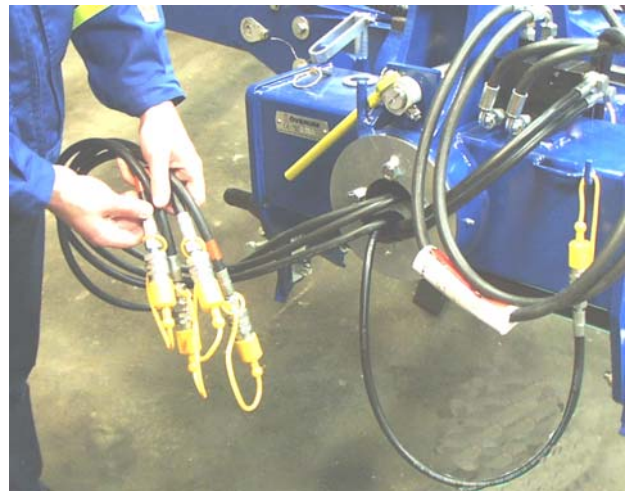
19. Dismount the male quick couplings from the hoses and put them through the turn over arm. Mount the quick couplings and make sure that the restrictor washers are properly mounted.
