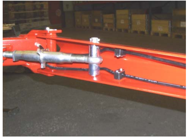
18. Bolt the hoses with clamps according to the picture above.
