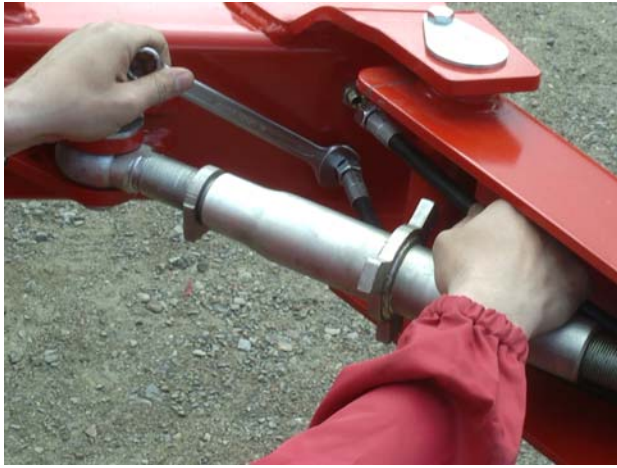
17. Mount the hydraulic hoses to the unions mounted in the front arm.
