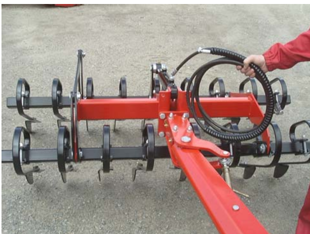
15. Mount the hydraulic hoses from the cylinder forwards to the unions.
